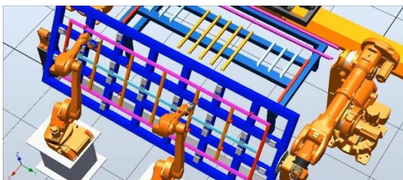
Figure 14: Two robots weld the far points
