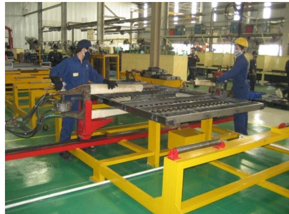
Figure 2: Two workers with spot welding gun
