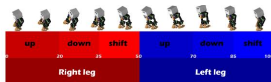
Figure 6: The Static Walking Sequence
