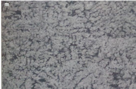
Fig.1 (b) Microstructure of 7SF (Al5083+5%SiC+2%Flyash)
