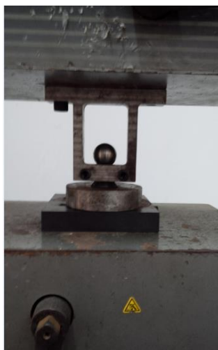
Figure 6: Tensile test for determination of resistance to static load of the femoral head
