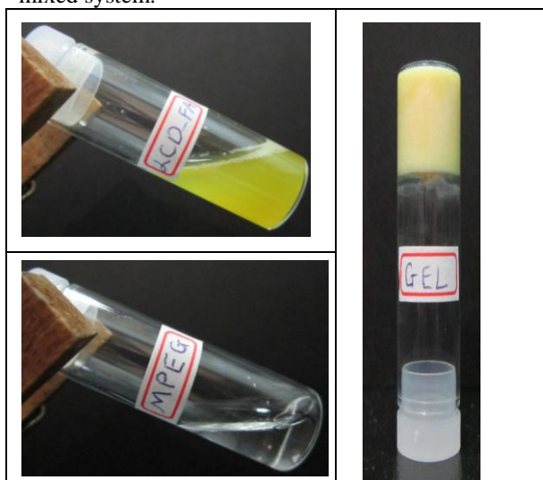
Figure 3 Photographs of the process of supramolecular hydrogel formation in an MPEG/ \alpha -CD-FA system.
