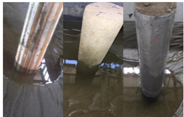
Figure 6: Difference in scour depths for wooden, concrete and steel obstacles
