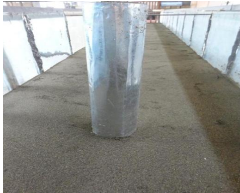
Figure 3: Obstacle made of Steel
