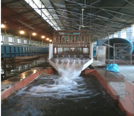
Figure 5: Discharge measurements with the help of a weir at the end of flume
