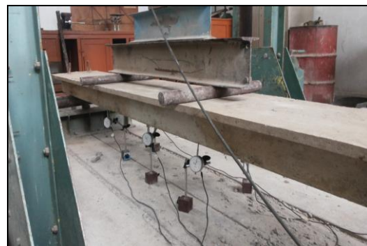
Figure 6: Loading setup for recording of deformation
