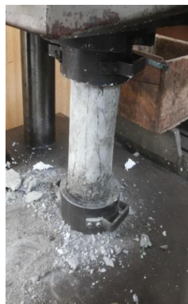
Figure 2: Concrete specimens testing in lab
