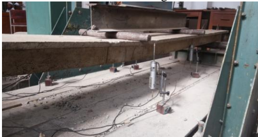
Figure 7: Ductile behaviour of panels when loaded
