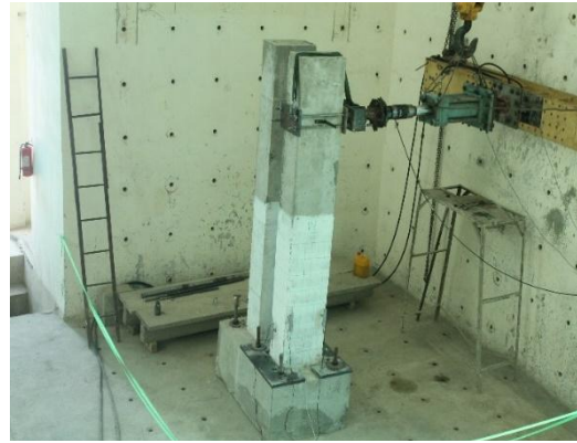
Figure 2: Specimen Construction & Setup
