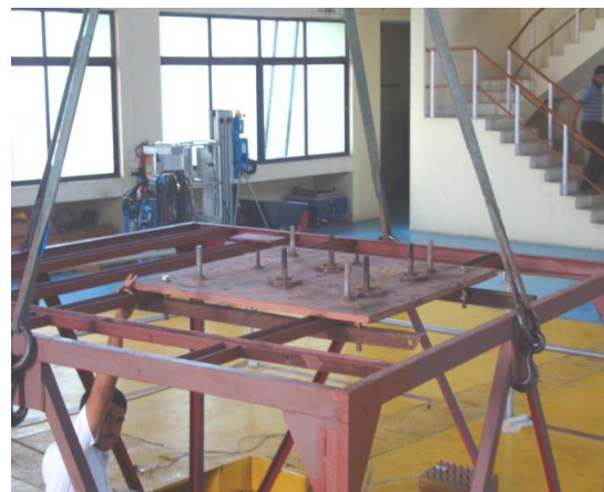
Figure 5: Steel frame with 0.275 Ton mass
