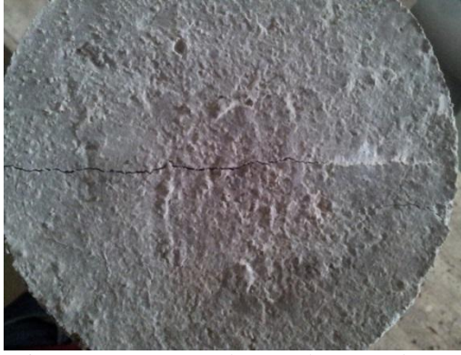
Fig 5: Specimen of Split Tensile Strength Test
