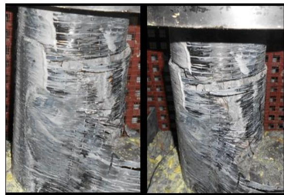
Figure 1. Cracking behavior of CFRP wrapped cylinders
