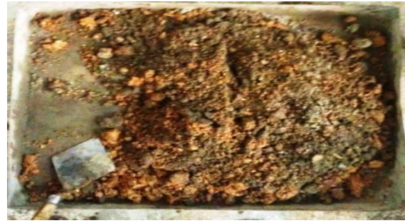
Fig. 1. A typical sawdust concrete mix with replacement level of 15%
