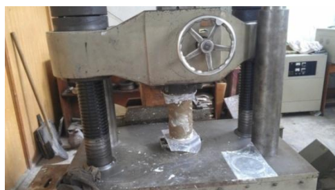
Fig. 2. Testing of Standard Cylindrical Specimen on UTM
