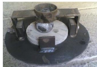
Figure 4 A Concrete sample arranged for Impact resistance test
