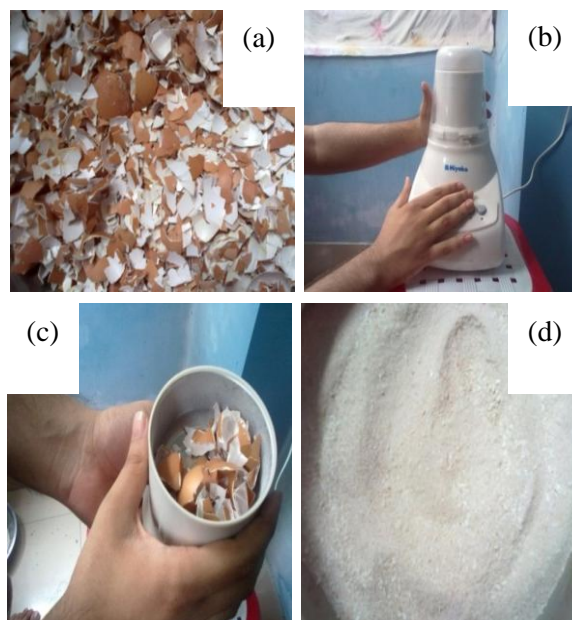
Figure 2: (a) Eggshell, (b) Blender, (c) Preparing for grinding, (d) Eggshell powder
