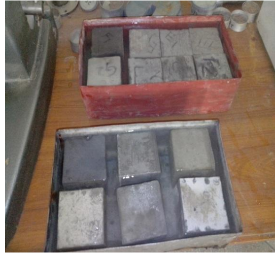
Figure 3: (a) normal water curing (b) steel containers for hot water curing in the oven
