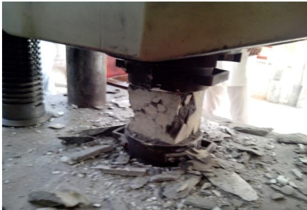
Figure 5: Compressive strength testing using UTM
