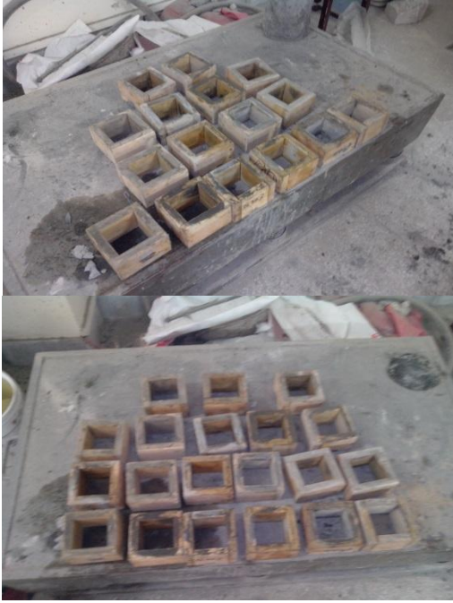
Figure 2: Wooden Molds prepared for casting RPC cubes specimens
