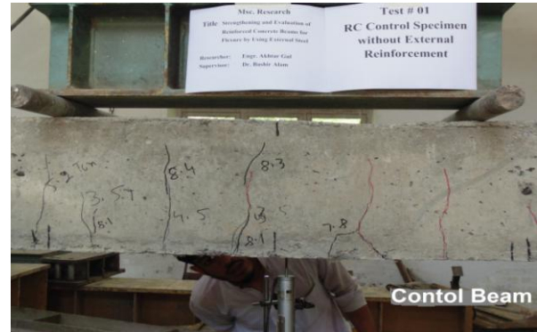
Figure: 06 Failure of Control Specimen TS1
