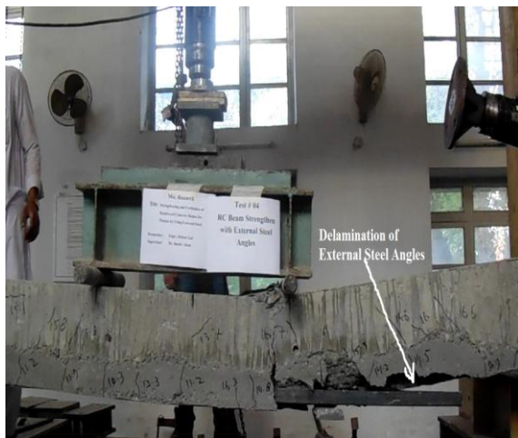
Figure: 09 Failure of Beam Strengthened with External Steel Angles
