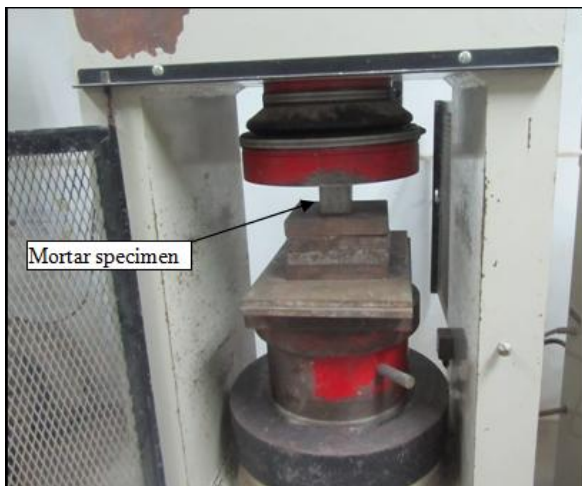
Figure 3: Compressive strength test of mortar cube
