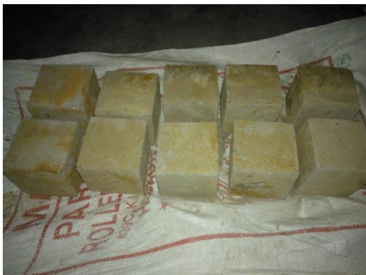
Fig. 1 Cubes after sulphate attack
