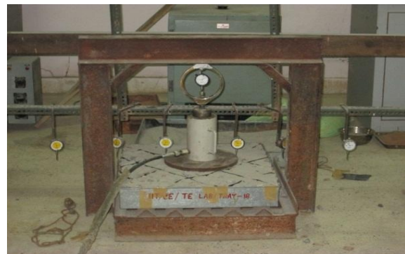
Figure 2. Experimental model for compressibility of Subbase
